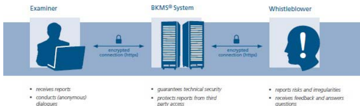
Figure 2: Security concept of the BKMS® system
